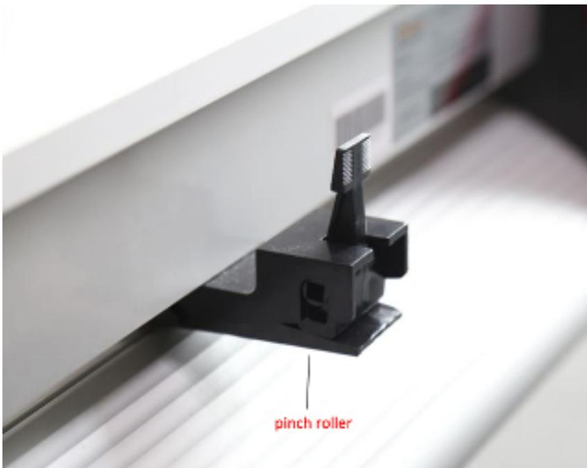
4.2.2.2 Insert the media into the space between the pinch roller and grit roller, and pull out media to the appropriate length at the front.
